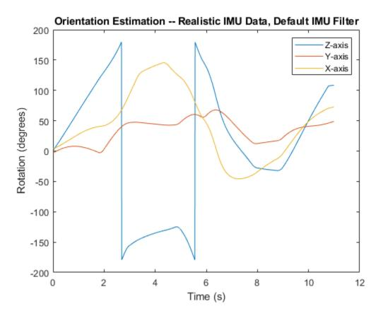
The ability of the imufilter to track the ground-truth data is significantly reduced when modeling a realistic IMU. To improve performance, modify properties of your imufilter object. These values were determined empirically. Run the loop again and plot the orientation estimate over time.
