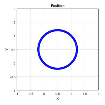
The trajectory output now appears circular. This is because the waypointTrajectory System object<sup>™</sup> minimizes the acceleration and angular velocity when interpolating, which results in smoother, more realistic motions in most scenarios.
