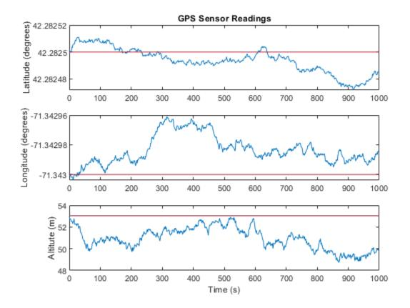
The position readings have noise controlled by HorizontalPositionAccuracy, VerticalPositionAccuracy, VelocityAccuracy, and DecayFactor. The DecayFactor property controls the drift in the noise model. By default, DecayFactor is set to 0.999, which approaches a random walk process. To observe the effect of the DecayFactor property:
