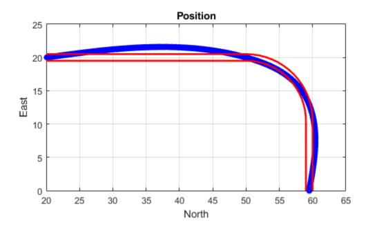
To create a trajectory within the bounds, add additional waypoints. Create a new waypointTrajectory System object<sup>™</sup>, and then call it in a loop to plot the generated trajectory. Cache the orientation, velocity, acceleration, and angular velocity output from the trajectory object.
