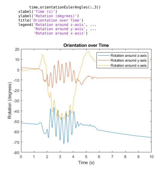
In the IMU recording, the shaking stops after approximately six seconds. Determine the resting orientation so that you can characterize how fast the ahrsfilter converges.
