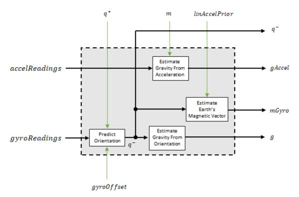
The orientation for the current frame is predicted by first estimating the angular change from the previous frame:
