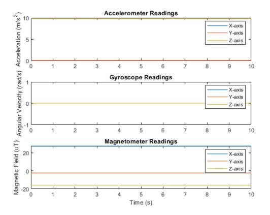
Orientation is not specified and the ground-truth motion is stationary, so the IMU sensor body coordinate system and the local NED coordinate system overlap for the entire simulation.
