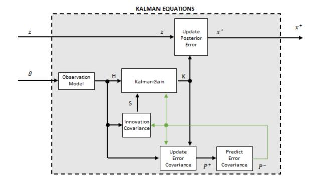
The observation model maps the 1-by-3 observed state, g, into the 3-by-9 true state, H. The observation model is constructed as:
