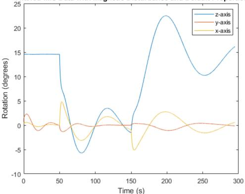
Filtered IMU Data with Magnetic Disturbance and Default Properties
