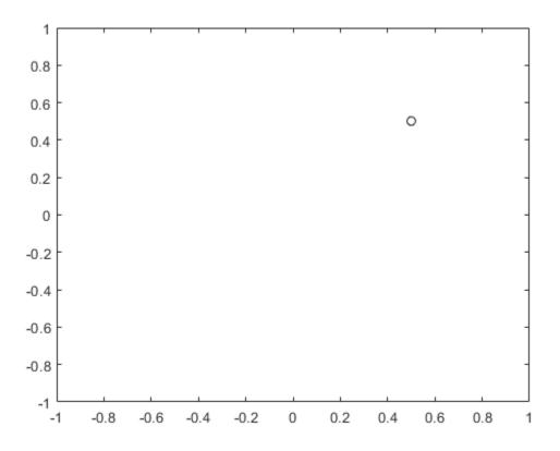
Create a quaternion vector specifying two separate rotations, one to rotate the frame 45 degrees and another to rotate the point -90 degrees about the z-axis. Use rotateframe to perform the rotations.
