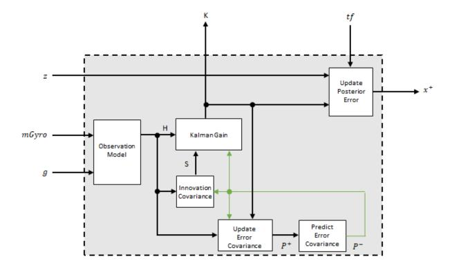
The observation model maps the 1-by-3 observed states, g and mGyro, into the 6-by-12 true state, H.
