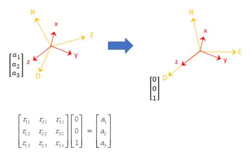
The third column of the rotation matrix corresponds to the accelerometer reading:
