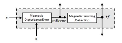
The magnetic disturbance error is calculated by matrix multiplication of the Kalman gain associated with the magnetic vector with the error signal:
