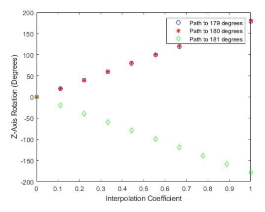
The path between q0 and q179 is clockwise to minimize the great circle distance. The path between q0 and q181 is counterclockwise to minimize the great circle distance. The path between q0 and q180 can be either clockwise or counterclockwise, depending on numerical rounding.
