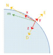
By definition, the *E*-axis is perpendicular to the *N*-*D* plane, therefore  $N \times D = E$ , within some amplitude scaling. If the sensor body frame is aligned with NED, both the acceleration vector from the accelerometer and the magnetic field vector from the magnetometer lie in the *N*-*D* plane. Therefore  $m \times a = y$ , again with some amplitude scaling.
