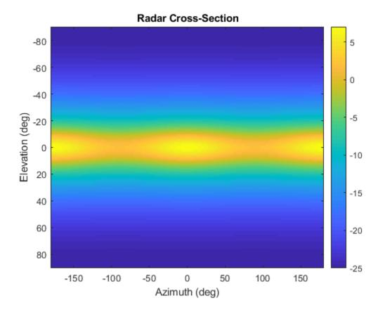
Create an <code>rcsSignature</code> object and plot an elevation cut at  $30^\circ$  azimuth.
