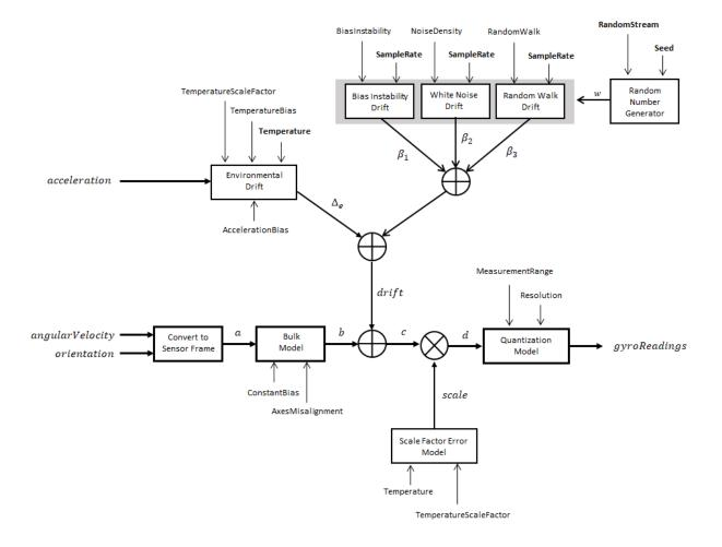
The ground-truth angular velocity is converted from the local frame to the sensor frame using the ground-truth orientation:
