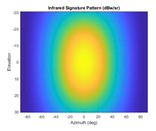
Get the IR intensity value at 25 degrees azimuth and 10 degrees elevation. value(irsig, 25, 10)
