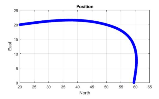
Inspect the orientation, velocity, acceleration, and angular velocity over time. The waypointTrajectory System object<sup>™</sup> creates a path through the specified constraints that minimized acceleration and angular velocity.
