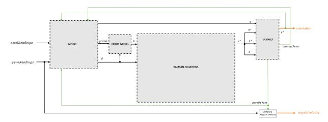
Before the first iteration, the accelReadings and gyroReadings inputs are chunked into 1-by-3 frames and DecimationFactor-by-3 frames, respectively. The algorithm uses the most current accelerometer readings corresponding to the chunk of gyroscope readings.
