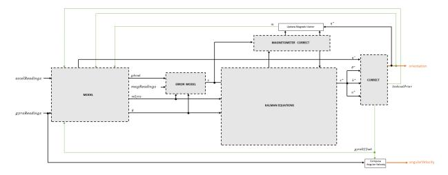
Before the first iteration, the accelReadings, gyroReadings, and magReadings inputs are chunked into DecimationFactor-by-3 frames. For each chunk, the algorithm uses the most current accelerometer and magnetometer readings corresponding to the chunk of gyroscope readings.
