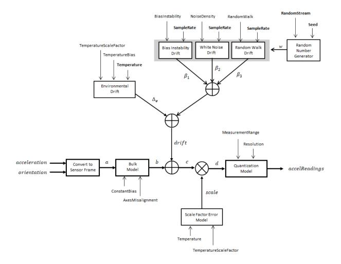
The ground-truth acceleration is converted from the local frame to the sensor frame using the ground-truth orientation:
