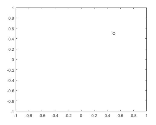
Create a quaternion vector specifying two separate rotations, one to rotate the point 45 and another to rotate the point -90 degrees about the *z*-axis. Use rotatepoint to perform the rotation.
