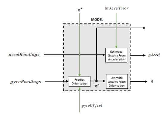
The orientation for the current frame is predicted by first estimating the angular change from the previous frame:
