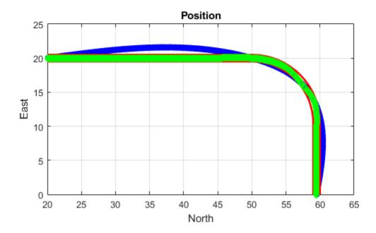
The generated trajectory now fits within the specified boundaries. Visualize the orientation, velocity, acceleration, and angular velocity of the generated trajectory.
