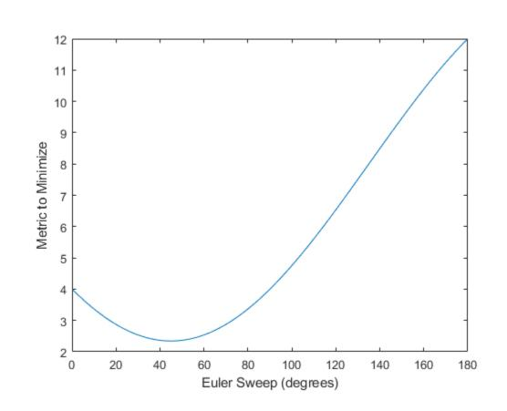
The minimum of the metric corresponds to the Euler angle sweep at 45 degrees. That is, meanrot defines the average between quaterion( $[0 \ 0 \ 0]$ ,'ZYX','frame') and quaternion( $[0 \ 0 \ 90]$ ,'ZYX','frame') as quaternion( $[0 \ 0 \ 45]$ ,'ZYX','frame'). Call meanrot with q0 and q90 to verify the same result.
