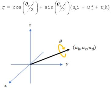
Given a quaternion in the form, q = a + bi + cj + dk, where *a* is the real part, you can solve for  $\theta_q$ :  $\theta_q = 2 \cos^{-1}(a)$ .
